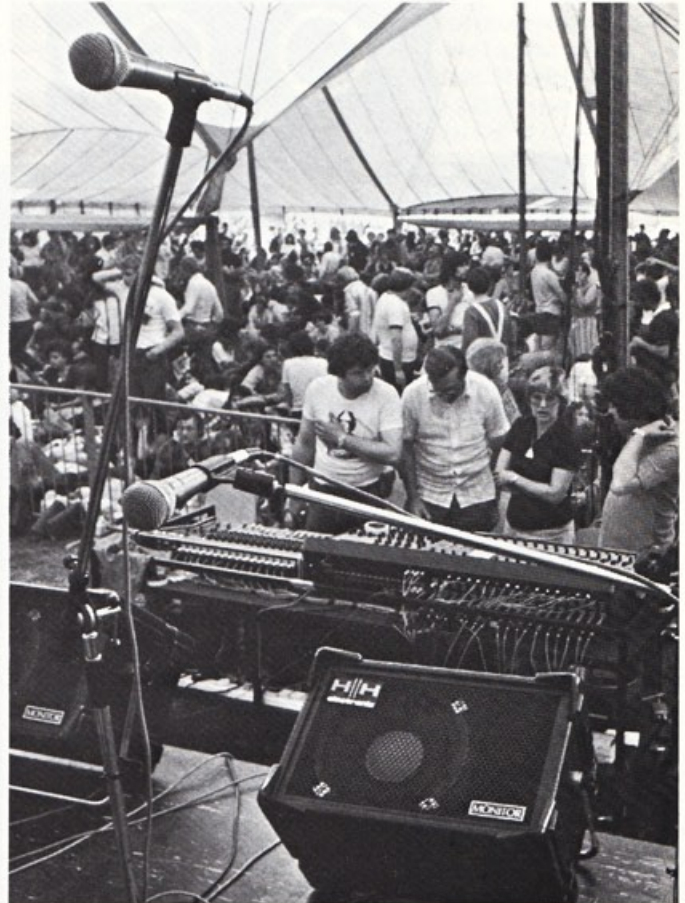
The Stereo-Six can readily link into a bigger main mixer thereby expanding the system.
